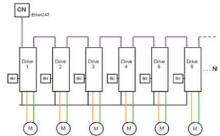
Traditional solution: one drive for each axis
